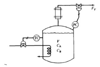
Assume  $F_V$ , is pure C. The reaction is first-order in  $C_A$ . The relative volatilities of A and C to B are  $_{AB}$ =1.2 and  $_{CB}$ =10. Assume perfect gases and constant pressure. Write the equations describing the system. List all assumptions.
